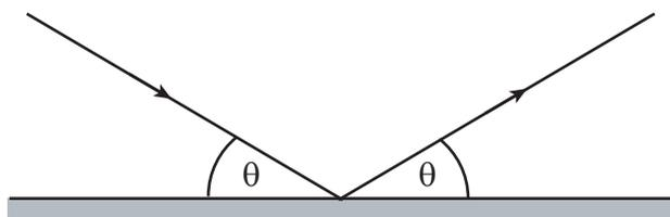
For a curved mirror, we must extend the law to say that the angles made by the incident and reflected rays with the tangent to the mirror must be equal.
